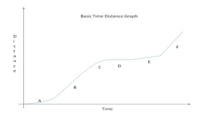
Curved lines represent acceleration. Section A of the graph shows the object speeding up (positive acceleration) while section C of the graph shows the object slowing down (negative acceleration). The steeper the line, the faster an object is going (the greater the acceleration). Section D shows that the objects speed is zero, section E shows the least acceleration and section F shows the greatest acceleration.
